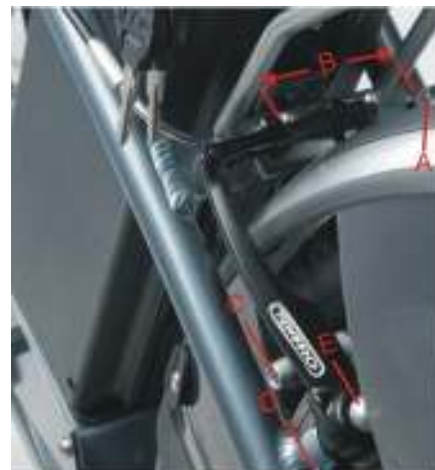
A-Cable clamp bolt B-No contact C-Pad fixing bolt D-Centering screw E-Arm fixing bolt
